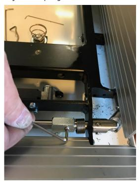
Drill holes and make thread for the fastening of the spring:
