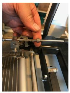
Hold the side-access-ramp in a  $90^{\circ}$  angle and tighten the two 6 mm socket screws with a 3 mm Allen key.
