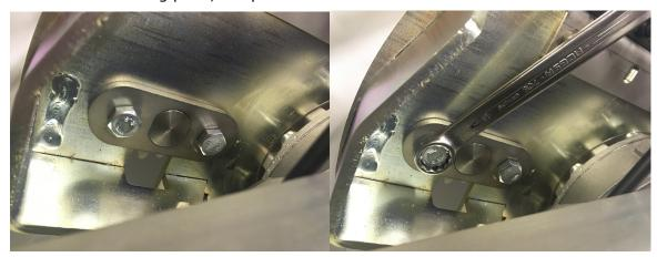
Use a 13 mm spanner to loosen the plate.
