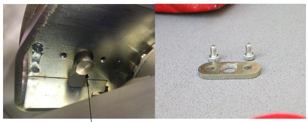
Pull out the shaft 2-3 mm
