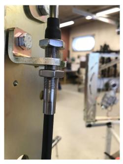
Push the cable up against the bracket and fasten the upper lock nut.
